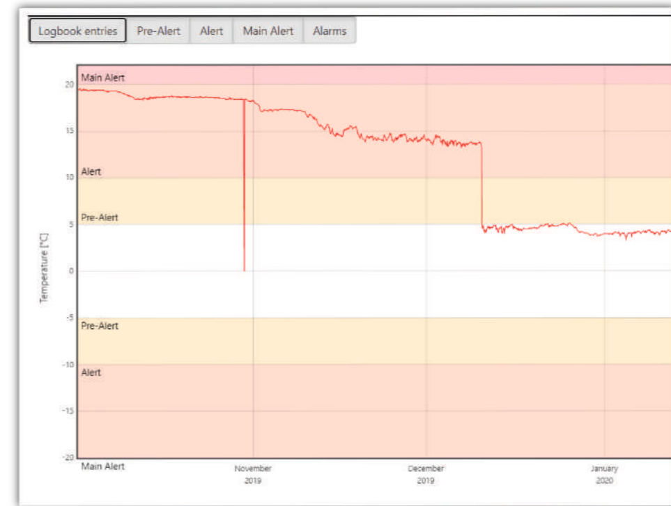
Alert limits in the measured value view
